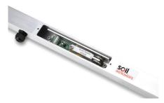
The Electrolevel Beam Sensor measures rotation of structures in the vertical plane.
